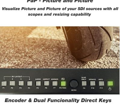
Encoder to easy navigate through the OSD menu, and direct keys with dual functionality (fixed/configurable). Activate [Fn] Mode to use F1 to F11 keys with your custom configuration and access your favourite adjustments just with a press. Keys LED lights can be turned off if required for dark environments.
