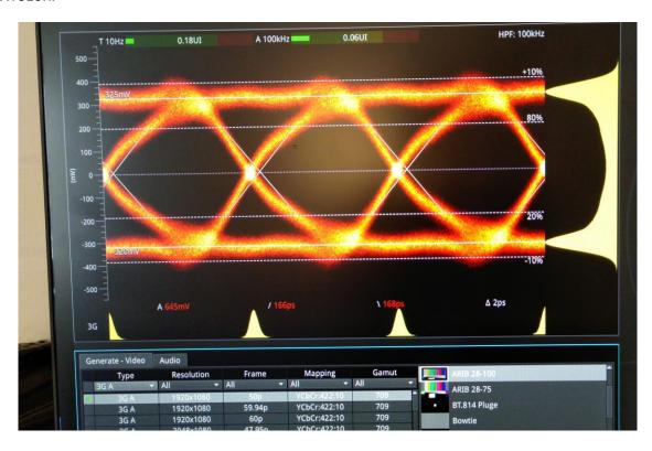
As is clearly visible, the L E N L3GGI04 product is very transparent to the 3G SDI signal, causing minimal distortion and the signal is still within the guide parameters
