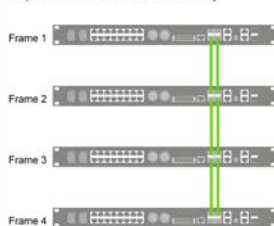
Four-frame ODIN system, duplicated IFL interconnectivity
