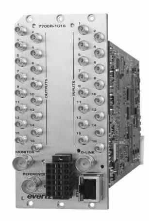
The 7700R16x16 is a small form factor router designed for critical applications where size is limited, whether for existing facilities who have run out of rack space or for trucks and vans. The 7700R16x16 uses up only 3 slots of a traditional Evertz 7700FR and has its own integrated controller. This means five 16x16 routers can fit in just 3RU.
