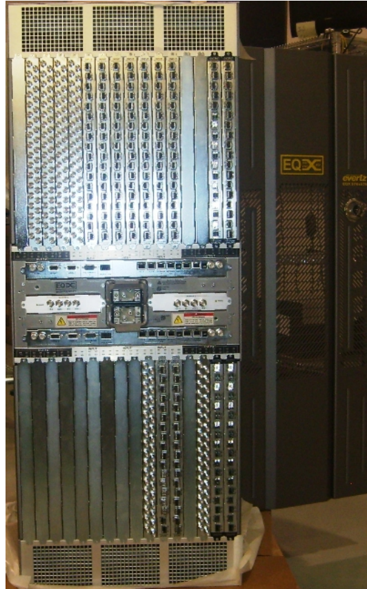
EQX Transmission System with Fiber I/O:
