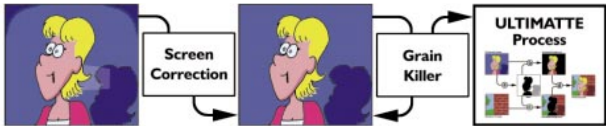
Fig. 2-1. The foreground image at left has an uneven backing: the upper corners are dark due to lens vignetting and a poorly painted patch appears behind the model. Using this image as input to the ULTIMATE process will result in a less-than-perfect composite. The SCREEN CORRECTION function can compensate for the flaws, producing an image with an even backing (center). If the image is noisy due to film grain or camera noise, the GRAIN KILLER function can filter the noise from the backing without affecting the foreground subject. After applying SCREEN CORRECTION and GRAIN KILLER , the image approaches the ideal conditions needed to achieve a perfect matte from the ULTIMATE process as described in Chapter One.
