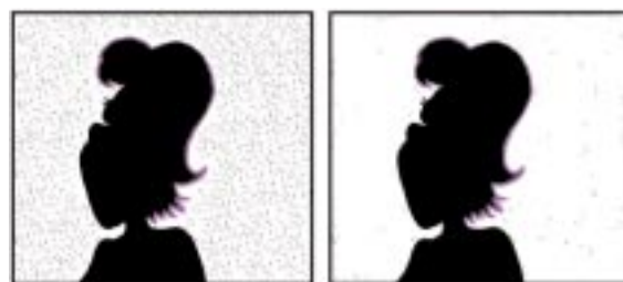
Fig. 2-9. The filter map before adjustment (left) and after (right). The map tells the Grain Killer logic where to filter the foreground image: areas that are white, corresponding to the unobstructed and shadowed backing, are filtered. Optionally in some systems, the transition areas (represented by a color) can also be filtered. Speckling of the image at left is caused by contamination of the backing due to film grain or camera noise. The user enters values which determine the limit between noise and fine foreground detail. At right, compromise values have been entered which eliminate most of the noise contamination while keeping the fine transition detail (color edge).
