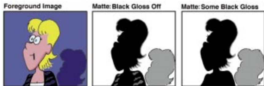
Fig. 3-2. Let's say our model is wearing a shiny black vinyl jacket which reflects some of the blue backing (left frame). The reflections show up as dark gray areas in the matte (middle frame) which will print through in the final composite. Advancing the Black Gloss control darkens these areas to black (right frame), eliminating print-through.
