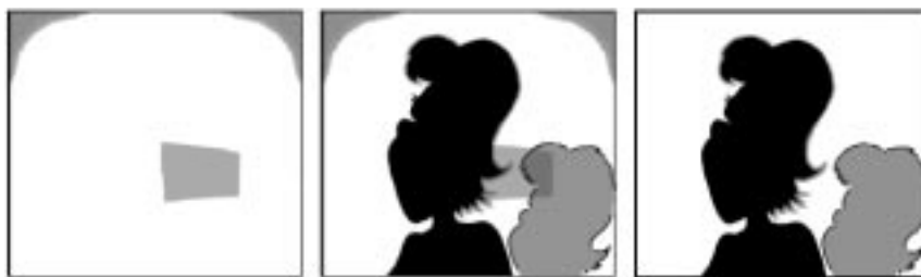
Fig. 2-7. Dividing the foreground matte (center) by the reference matte (left) yields the correction matte (right). Flaws in the backing do not appear in the correction matte, as if the matte were generated with an even backing (compare with Fig. 1-2).
