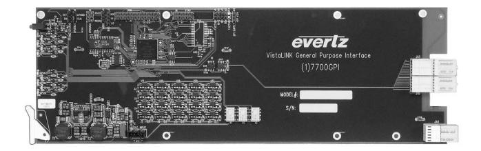
The 7700GPI VistaLINK™ General Purpose Interface module links third-party equipment and Evertz's VistaLINK™ Network Management System (NMS). Third-party equipment with fault alarming capabilities through General Purpose Interface outputs (GPO) can communicate fault alarm conditions to the VistaLINK™ application software through this GPO to SNMP translator thereby extending fault monitoring capabilities across the broadcast network.
